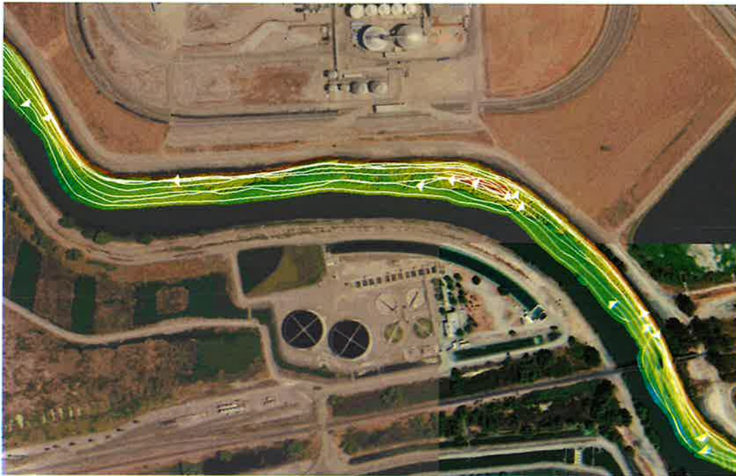
Figure 5-1. Multibeam survey lines shown in white over the bathymetric surface.
