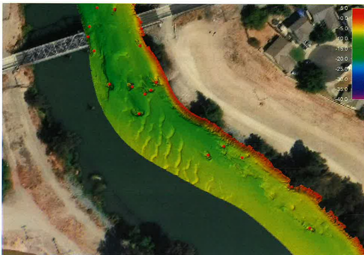
Figure 5-4 – Side-scan sonar contacts overlaid on the multibeam bathymetric surface.
